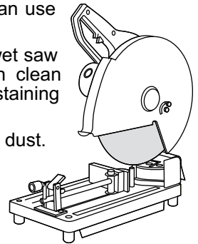
Chop saw with diamond blade
