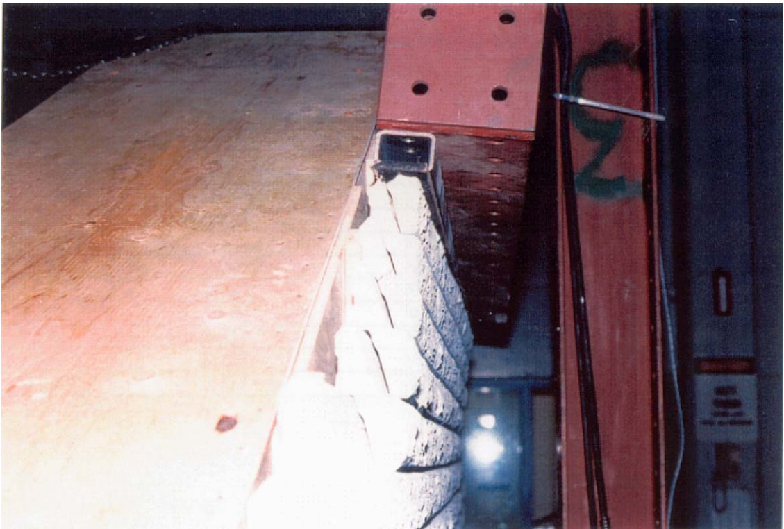
Figure 4.3 Condition of sample after shear test
