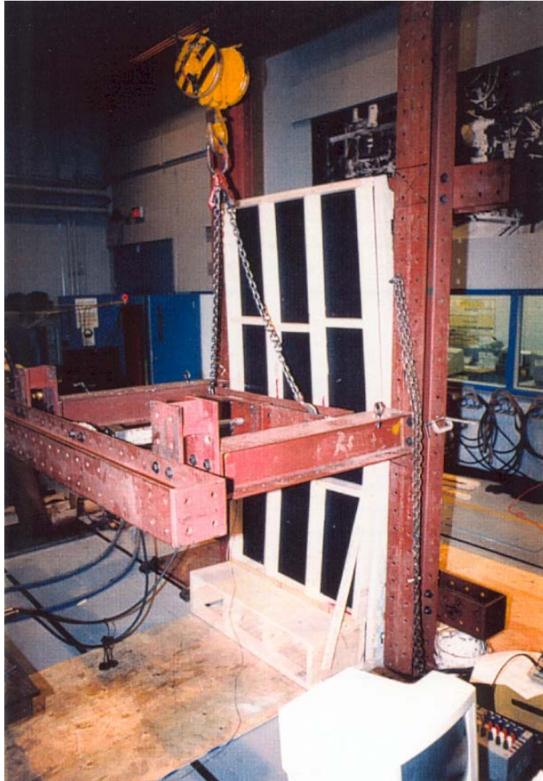
Figure 2.1 Test set-up for bending tests
