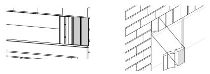
Note: If you need to cut a brick to fit the width of the opening, start installing soldiers at both ends and cut the brick in the middle of the opening. This will give a more symmetrical look.
